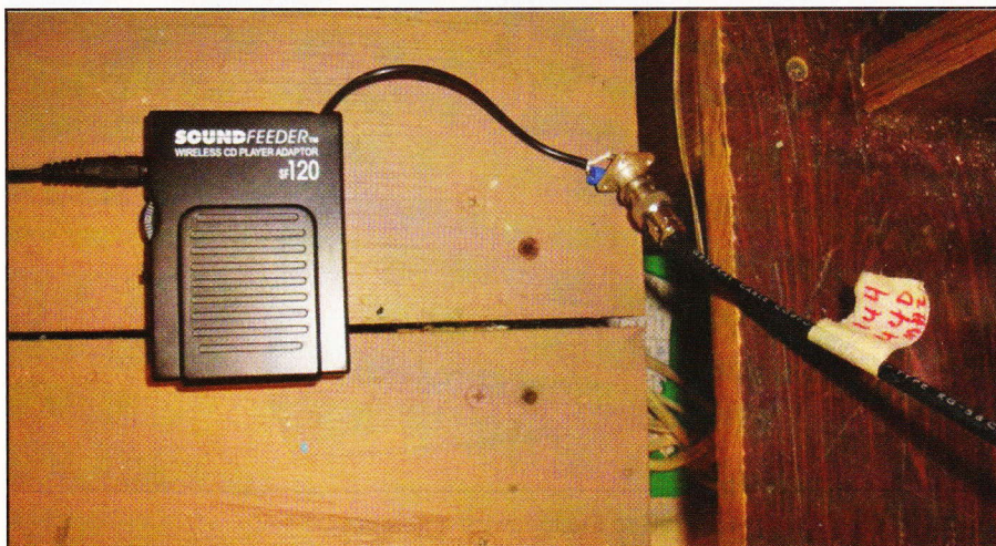
Photo C. The SoundFeeder FM transmitter is connected.
